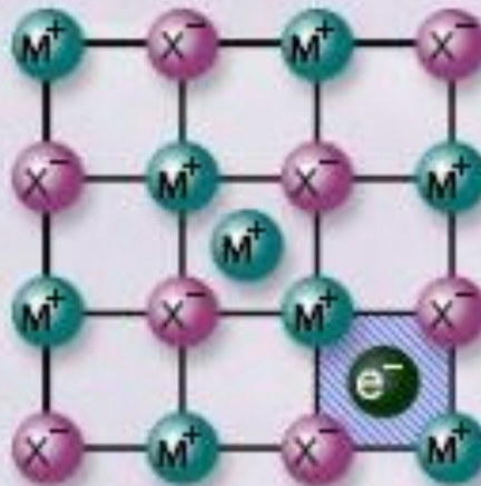
Metal excess defect due to interstitial cation
