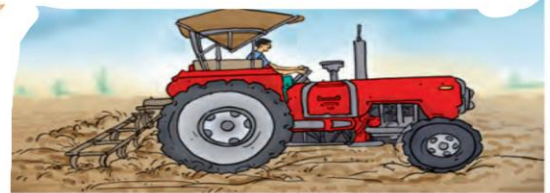
Fig. 1.1 (c) : Cultivator driven by a tractor
